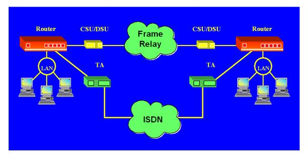
For our example we are connecting two routers using Frame Relay. This design will be sufficient for Frame Relay CIR's up to 128 Kbps. If you need more bandwidth than this, refer to the AHK Application Overview entitled "Disaster Recovery Strategy for T1 circuits using ISDN BRI". This document will discuss using Inverse Multiplexer in the place of Terminal Adapters to create virtual circuits up to 2 Mbps.
