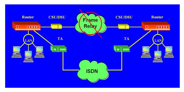
The Terminal Adapter "listens" for data by monitoring the Data Terminal Ready lead in the RS-232 or V.35 interface. This lead, or wire, only becomes energized when the router attempts to send data over the secondary path.
